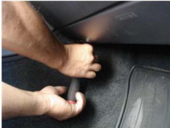
① Remove screws on Glove box.
