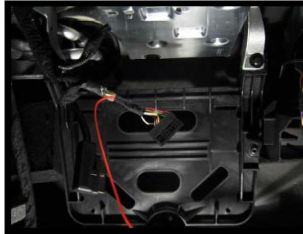
③ Connect Navi orange wire from Power cable to the 16<sup>th</sup> pin of the connector.
