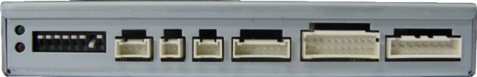
↑ LED    ↑ DIP S/W    ↑ Remote    ↑ MODE    ↑ IR OUT    ↑ RGB(IN)    ↑ A/V(IN/OUT)    ↑ POWER
