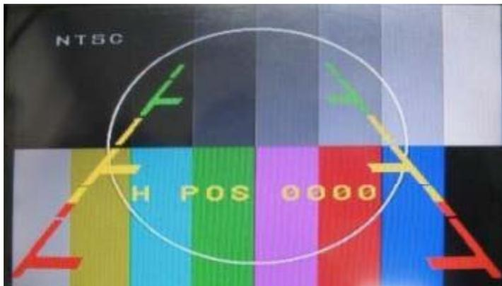
② After the setting done, rear parking guide line will appear in rear gear position. Once press "OK" button, "H\_POS" appears at the right and can adjust the line's position.
